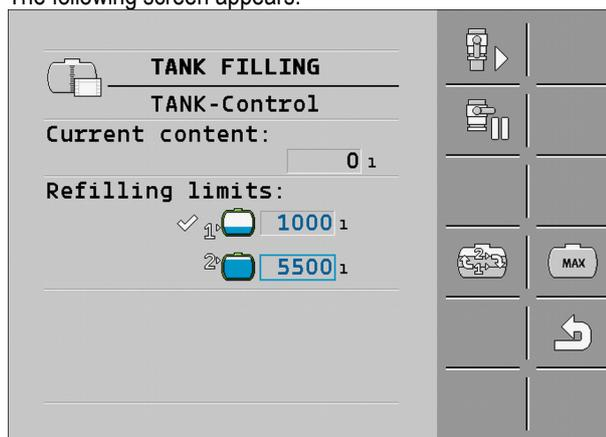
2. For refilling limit 1 and 2, you can enter up to two fill levels at which the filling pump should be stopped or the filling ball valve should be closed.
