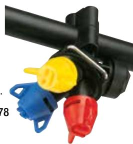
For mounting special nozzles such as the large drop flat spray nozzle and hollow cone nozzles, use the 322068 adaptor piece together with 3/8" union nuts.
