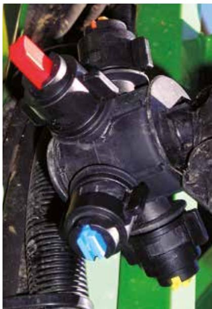
On sprayers with TeeJet or compatible systems use Single nozzles (**S**) and the 334862 black cap.
