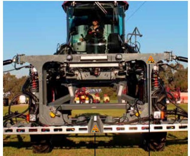
Rear mudguard: 97808104 Front paralift frame, in AutoHeight housing: 97813204
