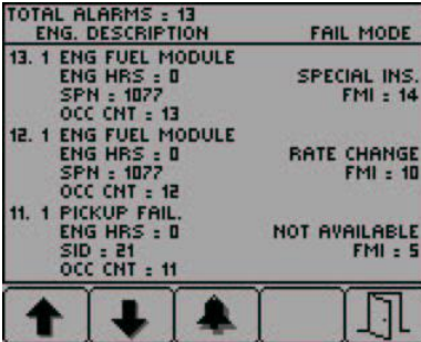
Figure 7.8.3: The alarm list screen, showing that alarm conditions have been acknowledged. Note that the exit key (key #5) has now been activated.
