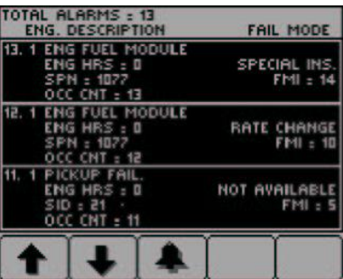
Figure 7.8.2: The alarm list screen, showing unacknowledged alarm conditions.
