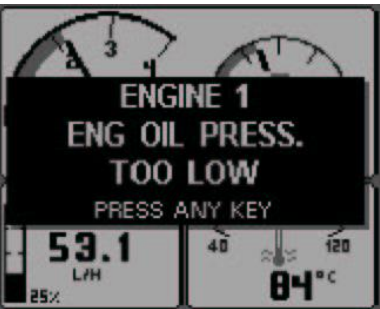
Figure 7.8.1: A representative alarm pop-up message, showing low engine oil pressure.
