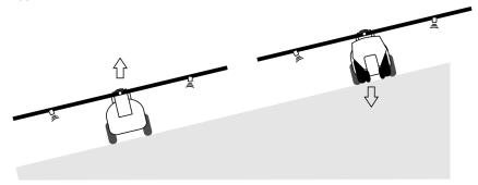
When turning on a slope, you can press a button to slope the boom in the opposite direction.
