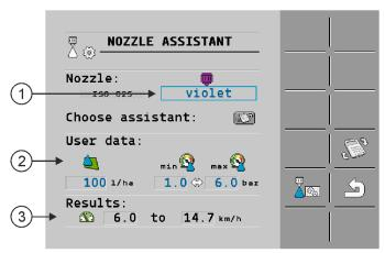
Determination of the fitting nozzles
