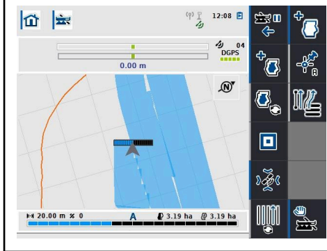
Automatic section control
