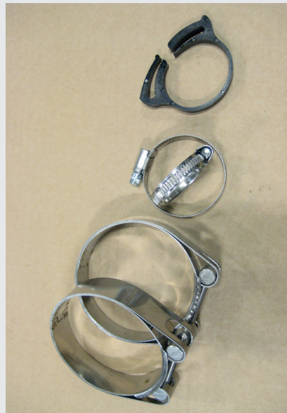
Hose clamps are all made of corrosion resistant material
