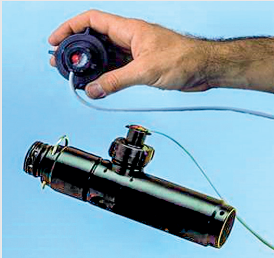
Flow housing and flow sensor showing LED at top
