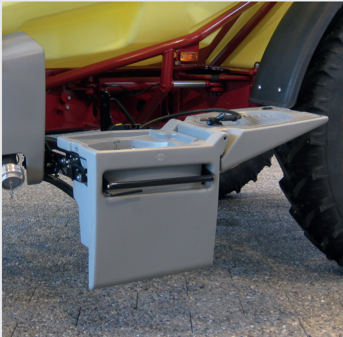
The TurboFiller is now integrated on COMMANDER models. Detail of swirl-plate at bottom of hopper
