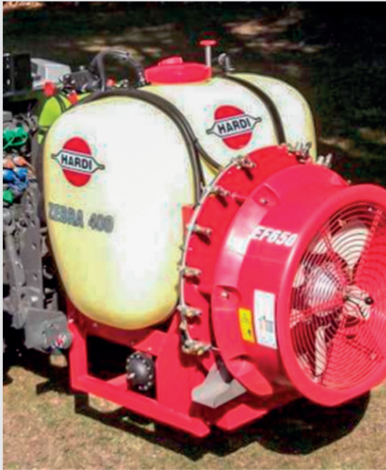
A lift-mounted axial blower
