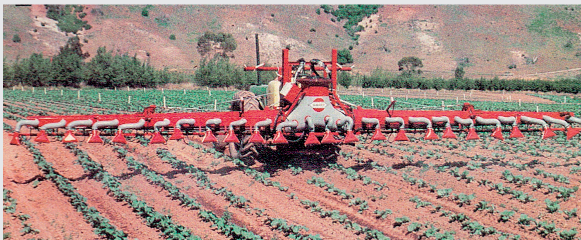
A 12 m (40ft.) Variant prototype from 1986 with 24 spouts
