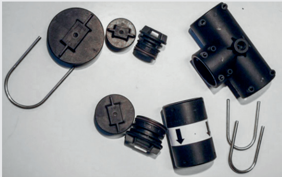
Plugs and tees to isolate liquid lines
