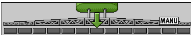
"MANU" means that DISTANCE-Control is deactivated and the boom must be raised and lowered manually.
