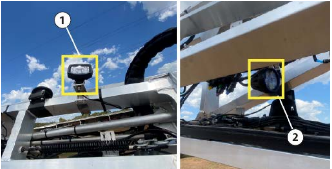
1. Over boom lights
