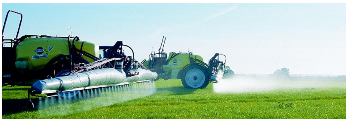
Wind from back of sprayer; slot angled back
