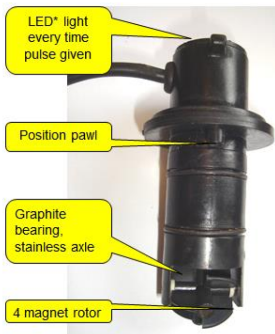
Flow sensor with rotor at bottom
