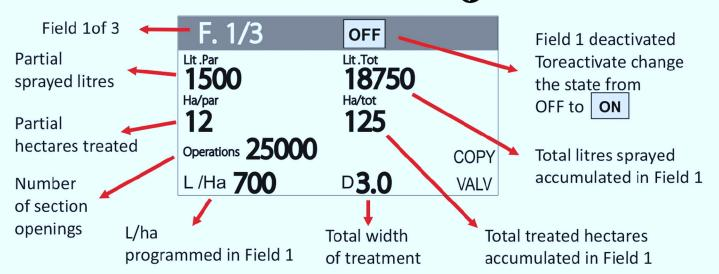
Press the button. The litres per hectare will be shown in a box. Press to make the value of litres per hectare go into edit mode. The value is modified digit by digit. To change the value use the buttons to increase or to decrease it. To switch from one number to the next one press or .To end press to save the new value. Finally, press to return to the main screen.
